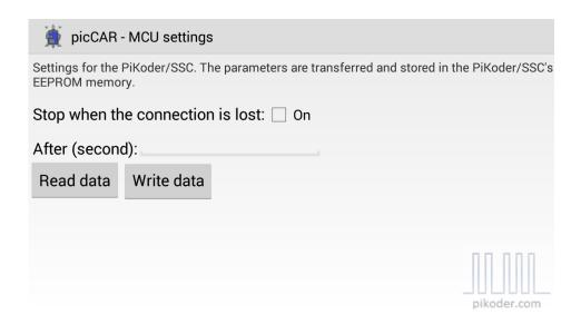
The picCAR app features a "fail-safe"-function (in combination with the PiKoder/SSC RX): if within a given time frame no new command would be received then all channels will be set to a neutral position. Since you can pre-program these neutral positions for your model (refer to <a href="PiKoder/SSC">PiKoder/SSC</a> RX User's Manual for mode details), you can ensure that a safe status is warranted (e.g. motors shut off).
