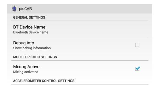
The default device name would be "HC-06" reflecting the PiKoder/SSC RX standard configuration. If you are employing another device then you can adapt the device name by tapping the field. Please note that the device which you are using has to be paired with your Android device.
