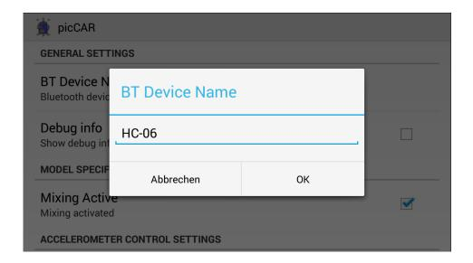
Mixing is a specific feature required to control "two motor models" such as tanks ("Mixing Active"); if your model requires a conventional control (one channel for direction, one channel for speed control), then uncheck the box.
