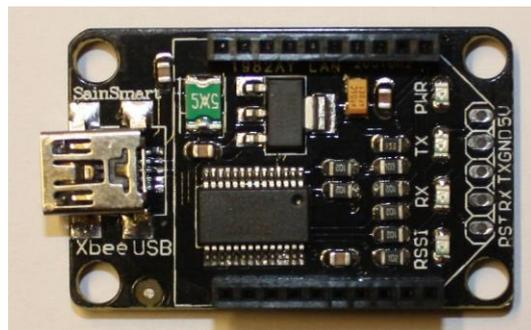
Then you would insert your XBee radio module into the connector of the adapter as shown below. After clicking the left most menu button with a “+” to add the first radio, a new window would appear allowing you to select the serial port to be used (see image on next page – in this instance it would be COM20). Select the port.
